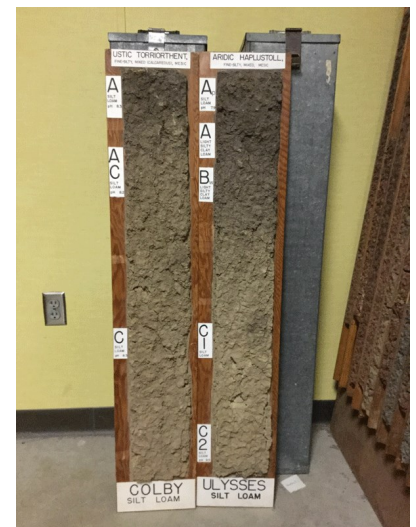
Figure 2. Side by side comparison of Colby and Ulysses soil monoliths. The Ulysses profile has a distinctively darker surface horizon that extends deeper in the profile compared to the Colby series. Photo by DeAnn Presley, K-State Research and Extension.
